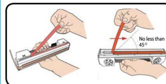
Remove the Printhead from its packaging. Gently remove the protective tape. Wet one of the included lint-free wipes with a good amount of de-ionized water and wipe the Printhead nozzles. Be careful not to wet the contacts.
