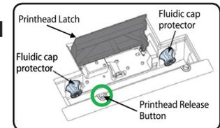
Remove the Fluidic Cap Protectors. Open the Ink Tank Door and release the Tank Latches. Insert the five ink tanks into their slots (latches are marked) label side up. Pull tanks back about an inch then re-insert to make a good connection. Close latches, ensuring both sides snap into place.
